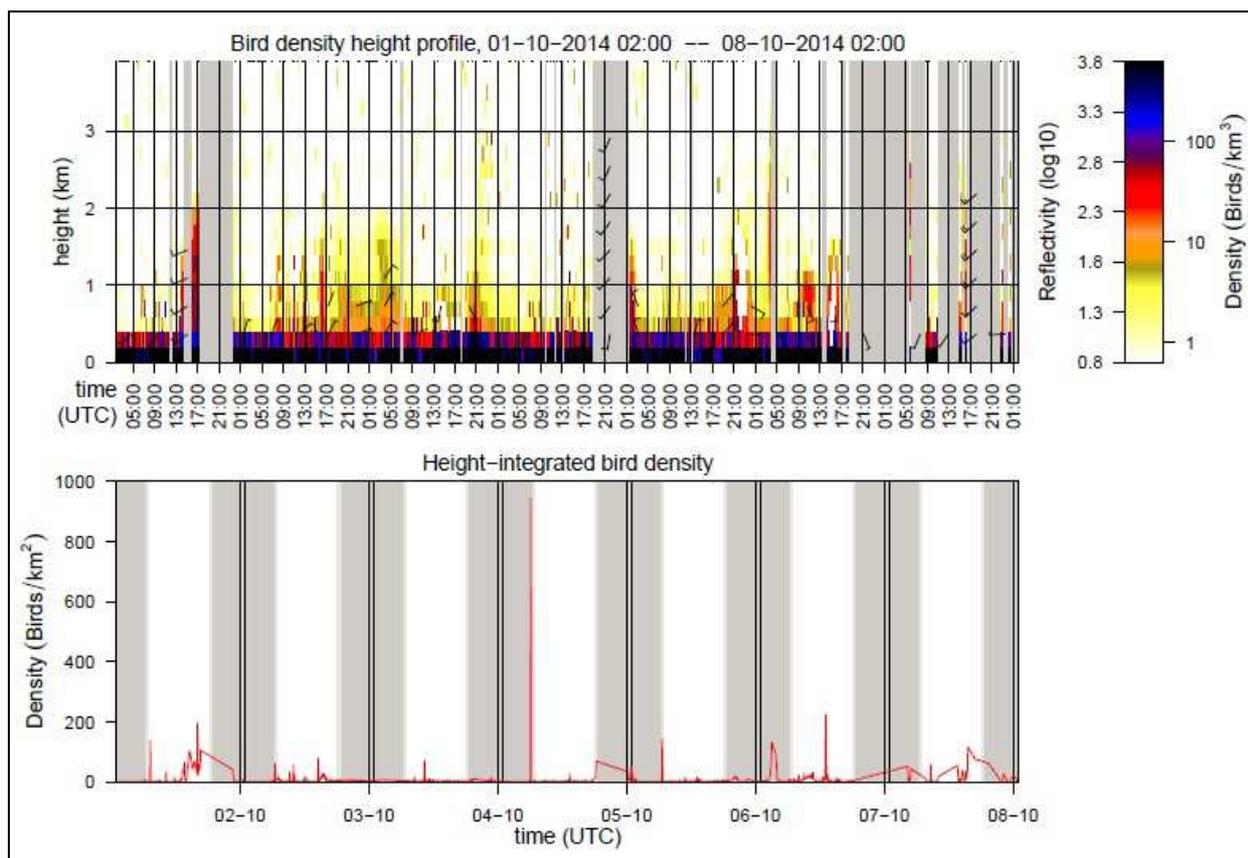
**Fig. 3.1.3:** Second rain filter applied on data from the radar Den Helder (The Netherlands) in the same week October 1-8, 2014. In this case the application of the rain filter was not completely successful probably due to the more scattered occurrence of rain precipitations and the lower values of bird density. A strong ground clutter is also evident between 0 and 500 m of altitude.
