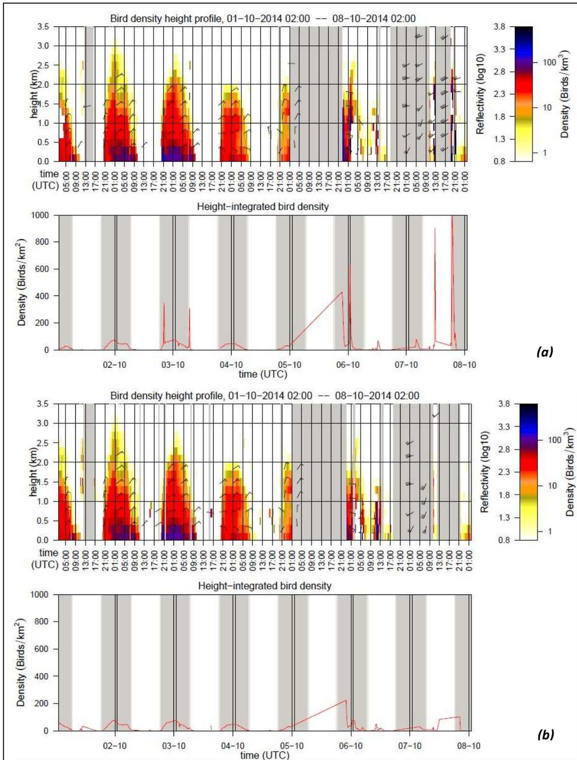
**Fig. 3.1.2:** Comparison of the effects produced by the two rain filters using data from the radar Wideumont (Belgium) in the week October 1-8, 2014. (a) First rain filter. (b) Second rain filter.
